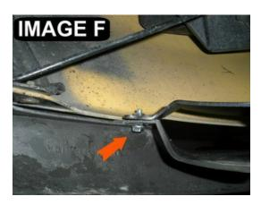
4. Install one of the supplied bolts and nuts. (IMAGE E) Tighten it down but not so much that you distort the look of the bumper or spoiler. (IMAGE F)
