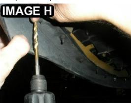
5. Now secure the inner portion of the air duct. There are no pre-existing holes so just eye ball it. (IMAGE G) Again, drill once, hold the two pieces together and make sure it looks good. Have your spare set of hands pull the lip back and drill as straight as possible. (IMAGE H)
