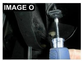
10. Locate the plastic screws in the upper section of your grill opening. (IMAGE N) There are three of them. You will remove the two outer ones and leave the center one. Take a short screw driver to remove the center screw. (IMAGE O)
