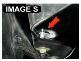
12. If you bend the plastic bumper cover down, (IMAGE R) you will see the hole in the hard plastic bumper as well. You will take the large washer on the SAE threaded bolt and drop it down from the top through the hole in the hard plastic bumper and bumper cover. (IMAGE S)
