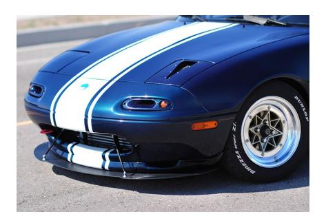
Thank you for purchasing the Track Dog Racing Radical Air Splitter. The Air Splitter is designed to help protect the factory R-Package lip by allowing the Air Splitter to slide over obstacles, such as steep driveways. The TDR Radical Air Splitter is made from 3/16" thick, high-impact ABS plastic and will surprisingly take a lot of abuse. The textured top finish blends in well with any color however; you might consider painting the R Spoiler for a nicer appearance such as the picture above.
